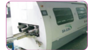
Wave Soldering Machines resolder the PCB after the process of insertion.
