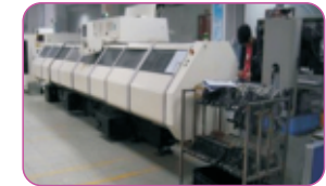
Surface mounting in progress is monitored by computerized control screen.
